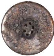
Injector before P.i. treatment.
