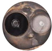
Cylinder head after one P.i. treatment.
